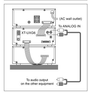
• By using audio cable (not supplied), connect between the audio output jacks on the other equipment and the ANALOG IN jacks.
